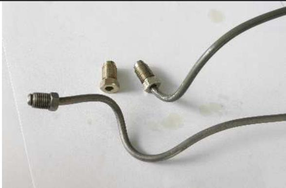
15. most RRS kits are supplied with a single flare tube nut style hose end which may require re flaring the original brake line and bending to suit. RRS has an optional braided flex line that will be compatible with a factory style double flare line end and 3/8 UNF tube nut
