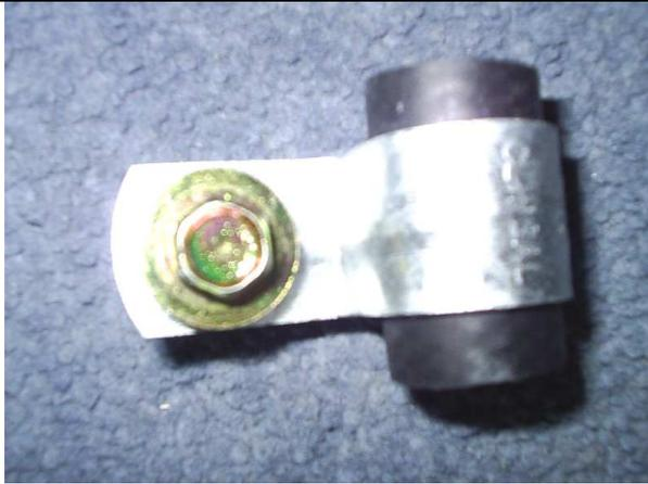
10. RRS supplies a park brake cable mounting clamp so that if there is a clearance issue resulting from the RRS conversion of the cable to any other vehicle components such as exhaust, the cable mounting clamp can be used to secure the cable to the chassis or floor panels
