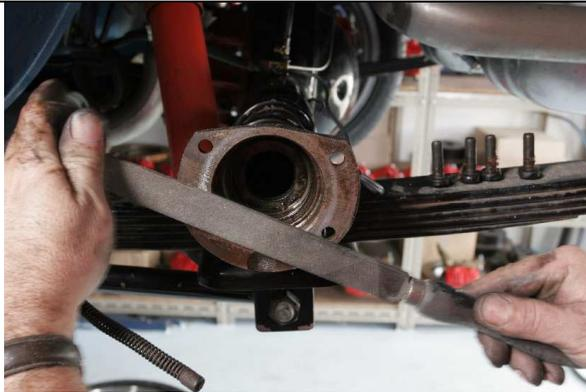
6. Remove axle assembly and backing plate. Check the axle seal and bearing for wear or leakage and replace if necessary. Check axle flange is free from burrs on the mounting face so that the RRS brake mounting plate fits squarely to the flange. Stamping flash is quite common on Ford axle housings and may require grinding or filing to neatly spigot into the CNC machined recess in the RRS brake mounting plate
