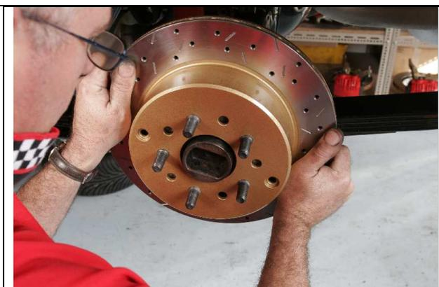
12. Fit the RRS disc, make sure the studs are fully engaged. The RRS supplied studs have longer shanks to accurately locate the new rotor. It is suggested that you use wheel nuts and washers to fully locate the disc on the axle. If the axle is in good condition and the disc is secure to the axle flange, the disc will run true.
