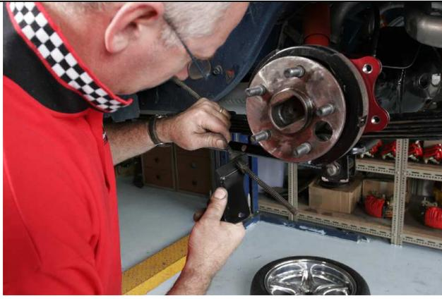
9. fit the RRS cable adaptor over the finger cone clip of your original park brake cable
