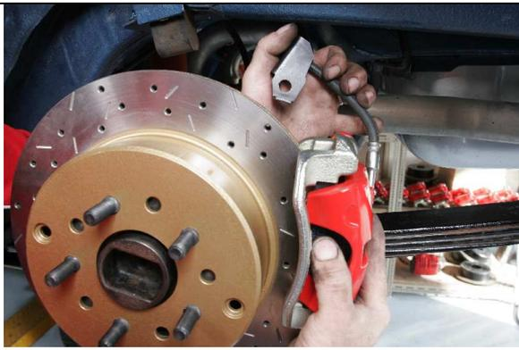
13. bolt the RRS caliper in place. Secure the flexible brake line so that adequate flex is maintained to allow for pad wear and caliper movement.
