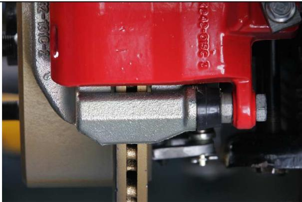
14. once the caliper is bolted in place, make sure the gap between the RRS caliper housing and disc is evenly spaced. If a misalignment occurs check that the disc is properly mounted, or the backing plate is properly mounted or alternatively consult with your nearest RRS supplier before road testing. NB do not shim or file to fit.
