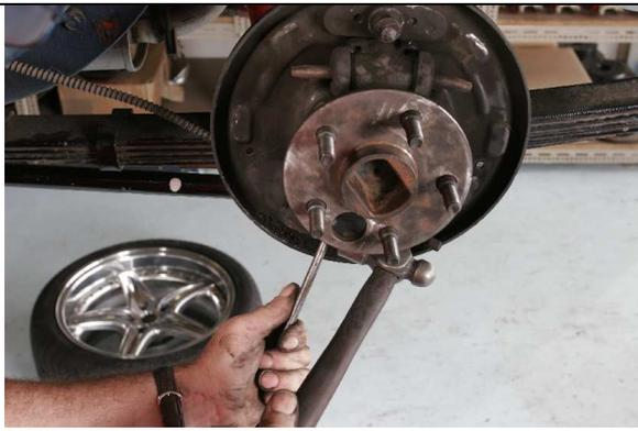
5. Remove park brake cable from backing plate. RRS suggest tapping a box wrench over the park brake cable finger cone clip, to make it easier to pull the cable through the backing plate
