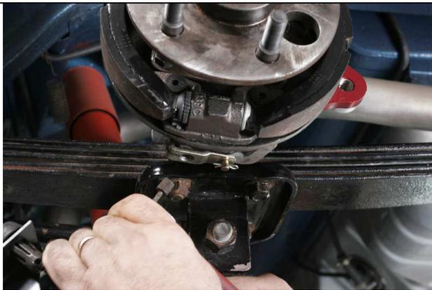
11. Fit factory cable end to RRS cable anchor. To make fitment easier, depress spring and hold with a pair of pliers. The RRS park brake mechanism will operate with all factory park brake cables regardless if it is foot or hand operated.
