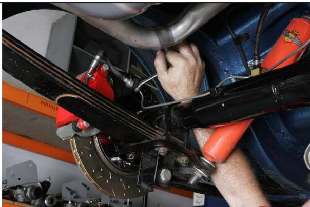
**Make sure brake line does not interfere with bump stop rubber.**
