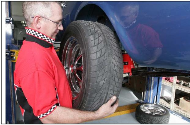
17. Fit the road wheels then check wheel nut tension. Follow normal brake bedding in procedures. Double check for fluid leaks and re-check wheel nut tension
