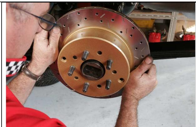
12. Fit the RRS disc, make sure the studs are fully engaged. The RRS supplied studs have longer shanks to accurately locate the new rotor. It is suggested that you use wheel nuts and washers to fully locate the disc on the axle. If the axle is in good condition and the disc is secure to the axle flange, the disc will run true.
