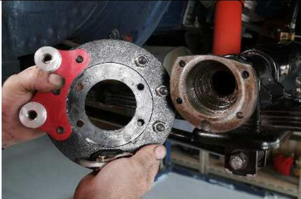
7. the spigot machined into the RRS mounting plate is clearly seen. Place the mounting plate onto the axle flange, making sure that it mounts flush to the axle housing by hand.
